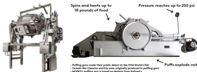
*Modern steamers (left) and gun puffers (right) used to make breakfast cereals. Intense steaming, drying and toasting ensures that the products are much the same a year or more after manufacture*
